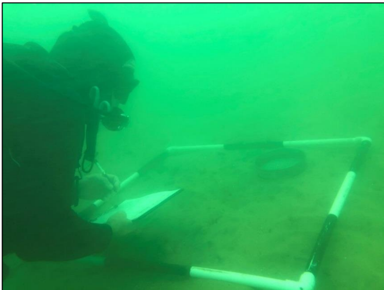
Quadrat with diver recording on a data sheet mounted on a writing slate.
