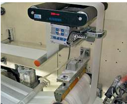
ELGUIDER DRS10 in Windelmaschine
