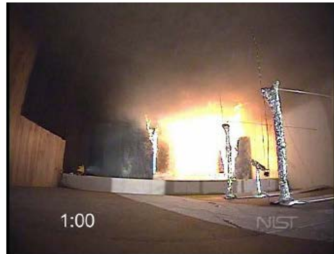
Figure 5-8. Flashover has occurred in alcove area, t = 60 seconds after ignition.
