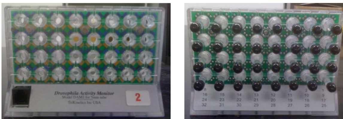
Figure 1a (left) and 1b (right). a) An example of a DAM, specifically model DAM2. The DAM2 connects to the computer and power source via the standard 4-wire telephone jack in the bottom left corner. b) Thirty-two individual flies are placed into tubes with an agar-sucrose food, covered with a black cap (shown), and capped off on the other end with cotton (not shown).
