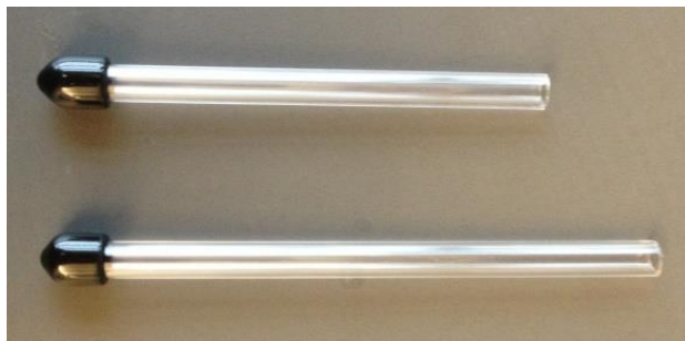
Figure 1. Left: A 5 × 65 mm polycarbonate tube with black cap (top) compared with a 5 × 80 mm tube (bottom). Right: When placed into a DAM, the 80 mm tube (right) has more room for motion compared to the 65 mm tube (left).
