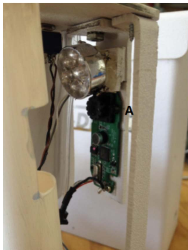
Figure 4. C270 HD webcam on L bracket. (A) Logitech C270 HD webcam with modified focus and removed IR filter.
