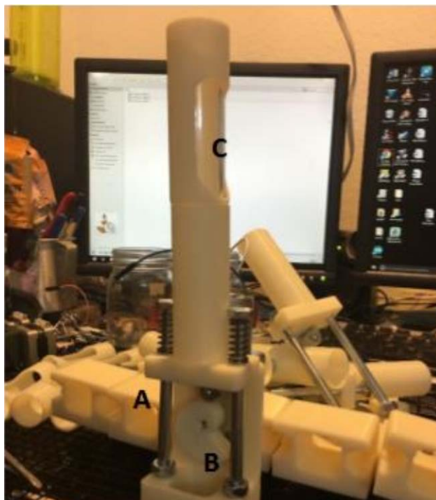
Figure 1. Motor cam and cylinder holder. (A) 4" × ¼" spring loaded bolts guide rails. (B) Snail cam with cabinet door roller. (C) Cylinder holder and viewing port.
