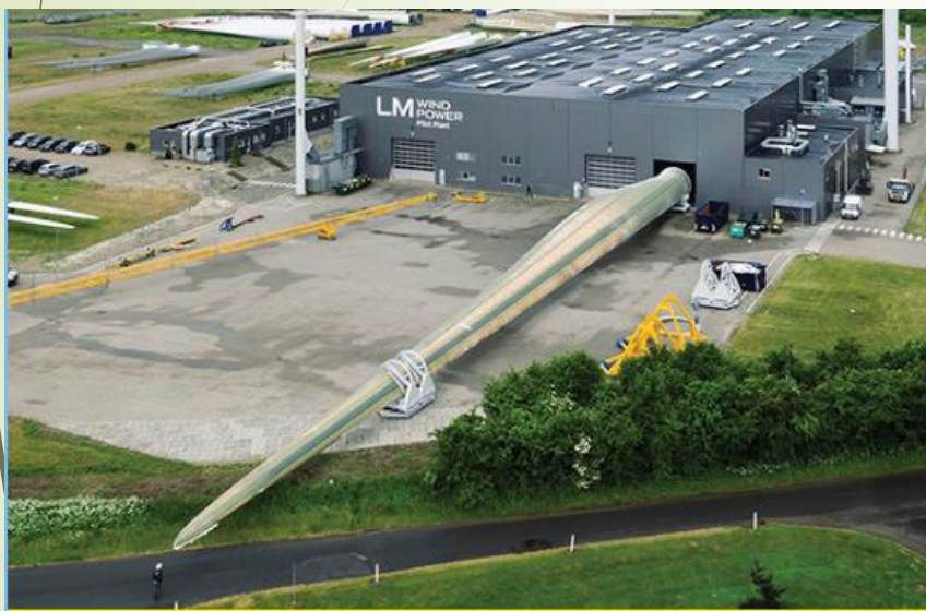
Currently the longest wind turbine blade is 88.4 metres, produced for an 8 MW offshore turbine. Photo: LM Wind Power, 2017
