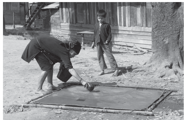
Fig. 6. Pouring the pulp on the mould in Ban Nam Leu village.
