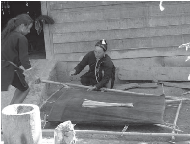
Fig. 4. Assembling the parts of a mould.
