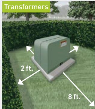
Planting closer than 8 feet from the front and 2 feet from the back and sides of pad-mounted transformers.
