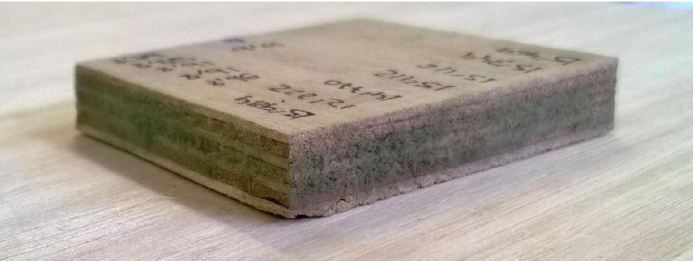
Thickness Swelling at Climate Chamber 90% RH T a = 23°C
