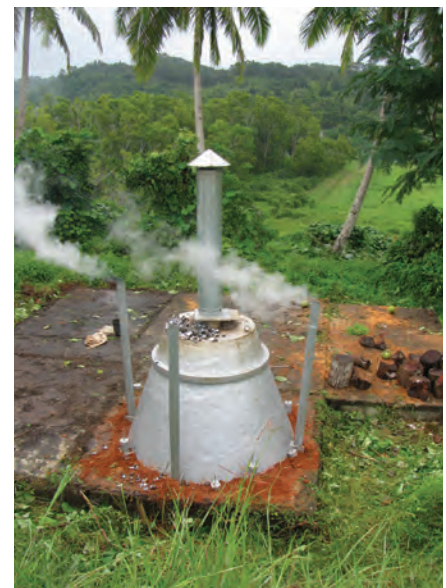
Biochar kiln in Naitasiri, Fiji: constructed by John Bennett from an old cement mix truck (Photo: Lex Thomson)
