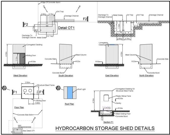
Plate 2-4: Proposed Fuel Storage Shed & Refuelling Pad
