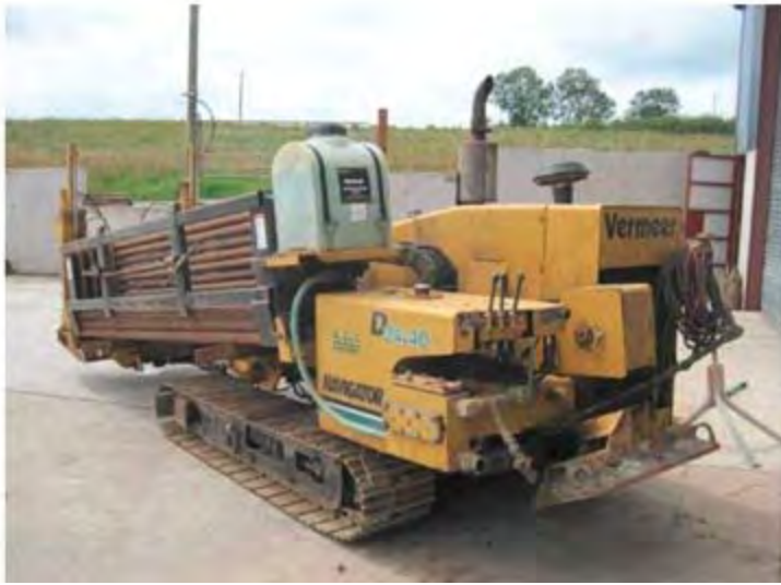
Typical Directional Drilling Rig
