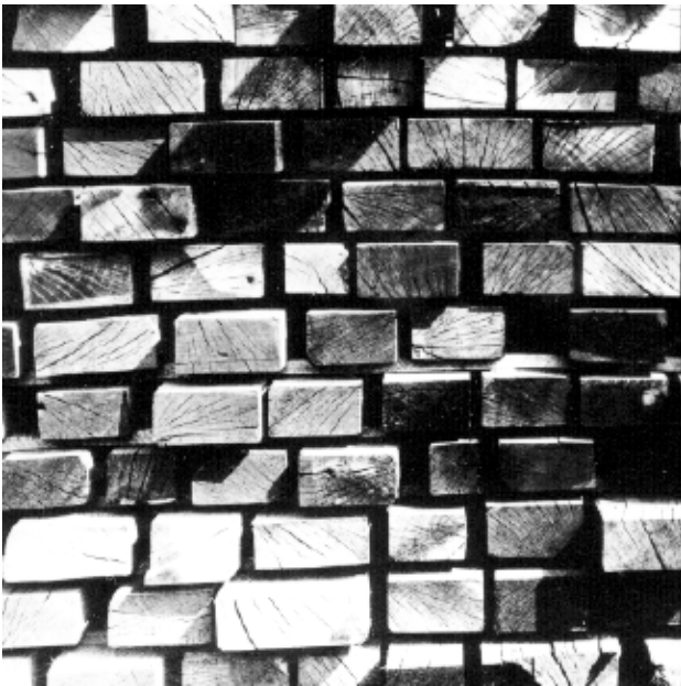
Figure 12-9. End checking in oak lumber.
