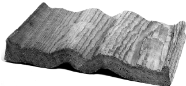
Figure 12-10. Severe collapse in western redcedar.
