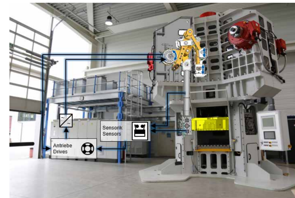
Figure Abstracted block diagram of the position control consisting of drives and sensors
