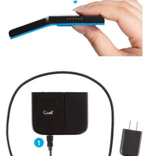
The AC Adapter should then be **plugged into a standard electrical outlet**. The USB connector on many computers is not powerful enough to charge Quell. The white indicator lights on the device will show that the device is charging. The number of lights shown will increase as the battery charges. When the battery is fully charged, all 5 lights will be lit. It will take approximately 3 hours to charge an empty battery. When the battery is fully charged, unplug the cable from the device.
