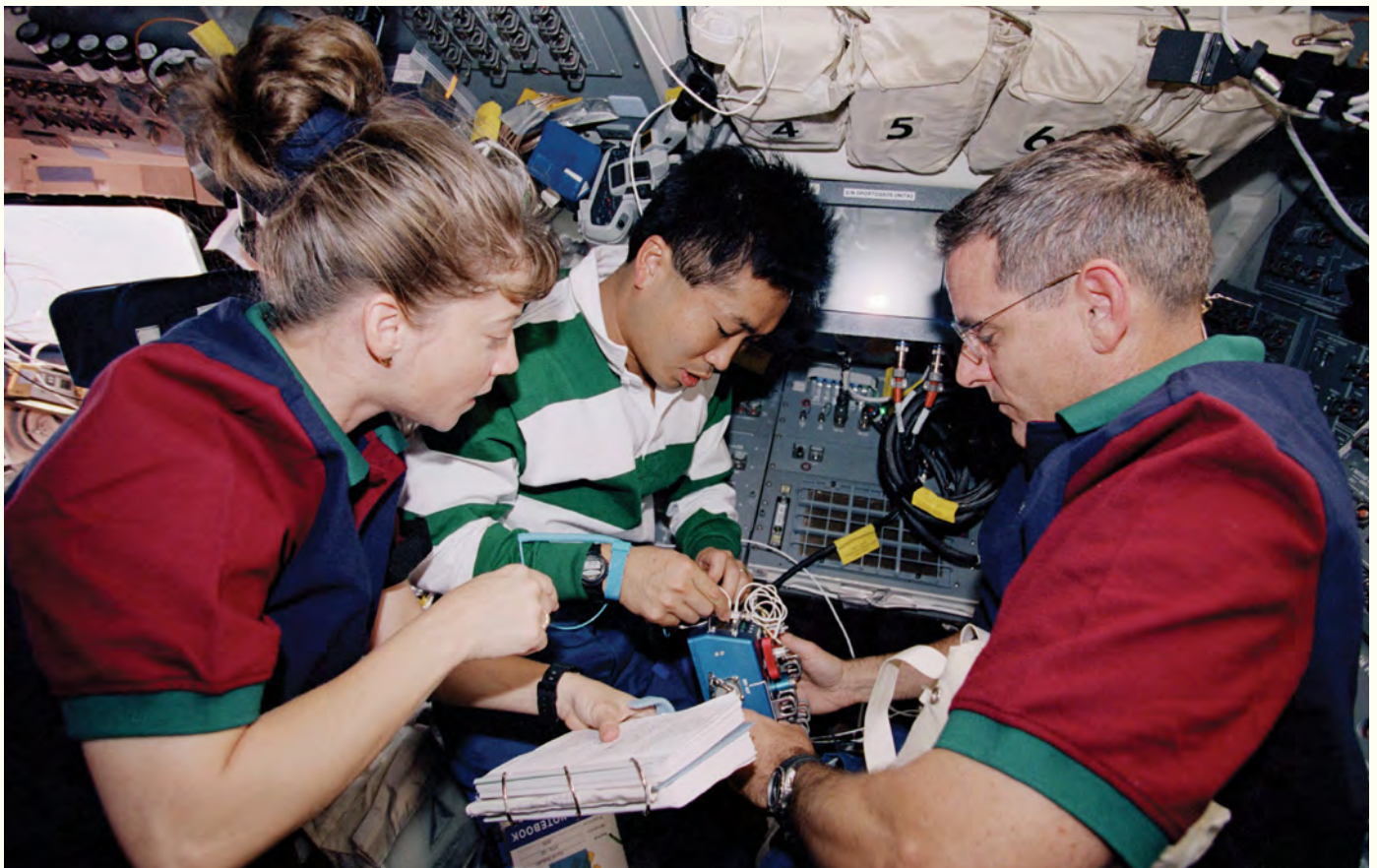
BELOW From the left, Pam, Koichi Wakata and William McArthur preparing a cable to bypass the tripped AC bus.
