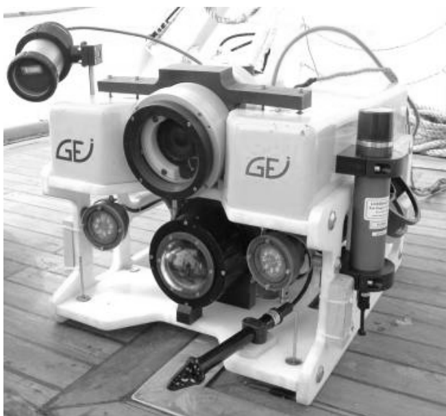
Fig. 2: ROV "Pollux" equipped with camera and strobe housing, grabber and acoustic transponder
