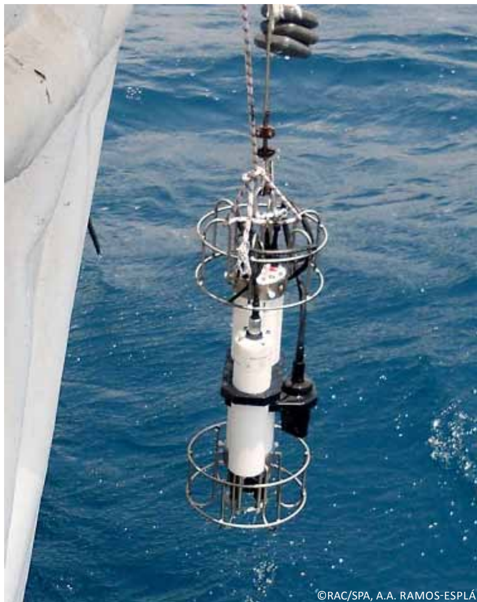
Figure 8. Launching the TCD off the stern of the oceanographic boat 'Cana'
