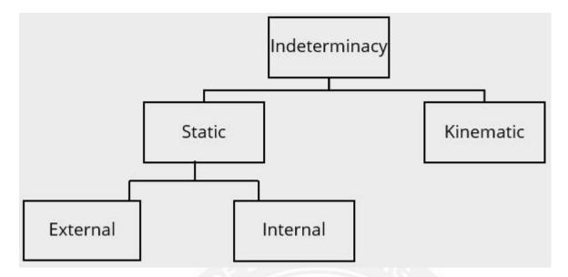
The degree of static indeterminacy or degree of redundancy shows the number of additional equations required to solve the system. External indeterminacy is related to the support system of the structure whereas internal indeterminacy is related to the internal stress in the members of the structure. The degree of kinematic indeterminacy shows the number of unknown joint deformations.
