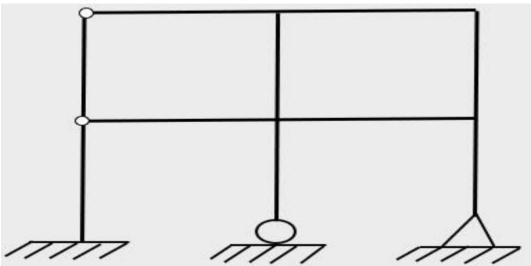
Degree of static indeterminacy = (3m+r) - (3j+c)= (3\*10+6) - (3\*9+3) since, c = (3-1) + (2-1)= 36 - 30= 6
