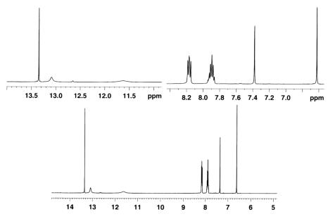
Fig. 8. <sup>1</sup>H-NMR spectrum of compound B of the ascidian *R. birkelandi* dissolved in DMSO-d<sub>6</sub>, conducted in an NMR Bruker Avance 500 MHz
