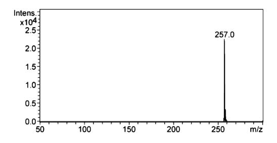
Fig. 6. Mass spectrum of compound B of the ascidian *R. birkelandi* conducted in an MS/MS Bruker Esquire 6000 with electrospray ionization in positive mode
