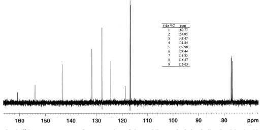
Fig. 3. <sup>13</sup>C-NMR spectrum of compound A of the ascidian *R. birkelandi* dissolved in CDCl<sub>3</sub>, performed on a NMR Bruker Avance 500 MHz
