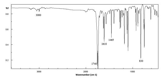
Fig. 1. Infrared spectrum of compound A of the ascidian *R. birkelandi* analyzed on the computer model Bruker IFS 66 V / S in a KBr pellet
