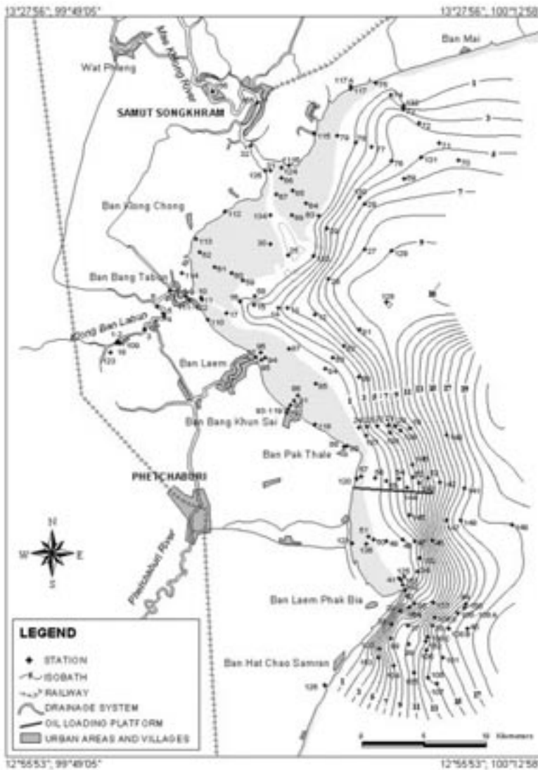
Fig. 3 - Digitalized map of the coastal area of Phetchaburi showing the bathymetric contours, the location of at sea and inland stations, and the extension of the tidal flat (shaded).
