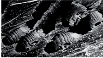
Fig. 309. Isopods Limnoria caused destruction to marine timber.
