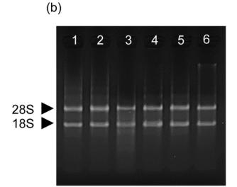
Gel electrophoresis results of six octocoral species: *Sinularia acuta* (1), *Lobophytum hsiehi* (2), *Stereonephthya* sp. (3), *Sclereonephthya* sp. (4), *Dendronephthya*sp. (5), and *Litophyton* sp. (6) in three replicates by using (a) CTAB/10%SDS RNA extraction and (b) on column RNA extraction
