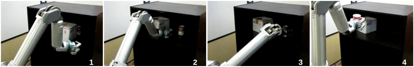
Fig. 16 An example plan to retrieve a can behind a large ungraspable box on a shelf. The robot first pushes the ungraspable large box to the side and then reaches in to get the can out.
