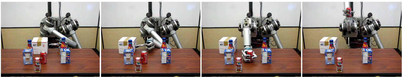
Fig. 1 The planner rearranging clutter to reach to a goal object. Pushing actions are useful for moving large objects that do not fit inside the hand, i.e. are not graspable. Planning time for the full sequence of actions in this example is 16.6 sec.
