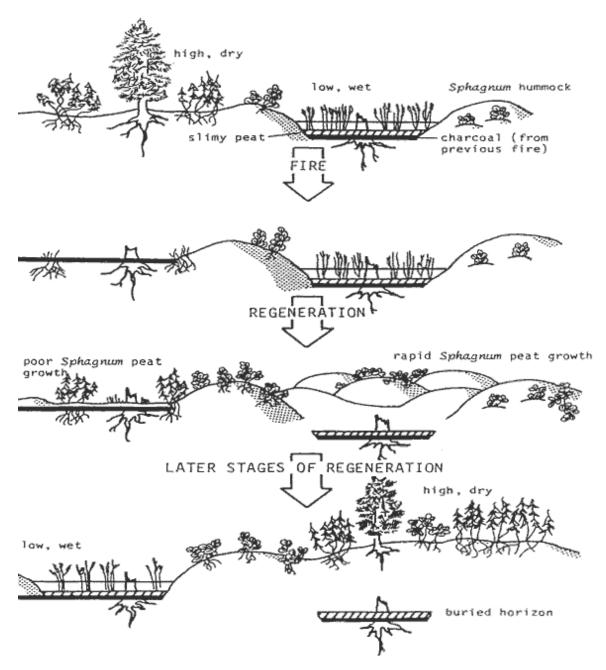
Figure 6.4: Fire induced hummock-hollow recycling. Source: Hebda 1977.
