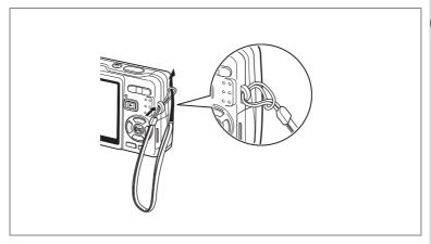
Pass the narrow end of the strap through the strap lug and pass the other end through the loop on the end of the strap.
