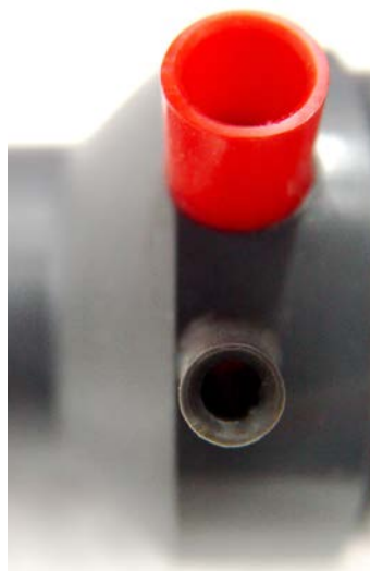
Nozzle with air- and ozon- plug
