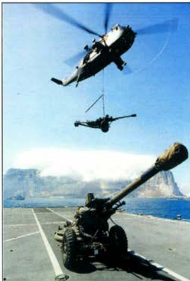
● GUNS: A Sea King helicopter from HMS Ocean transporting 105mm light guns ashore during Exercise Rock Wader.
