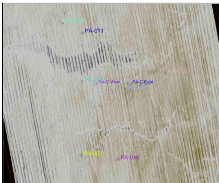
Figure 3-4. Time slice (data at equal time) through the 1997 PA 3D seismic data
