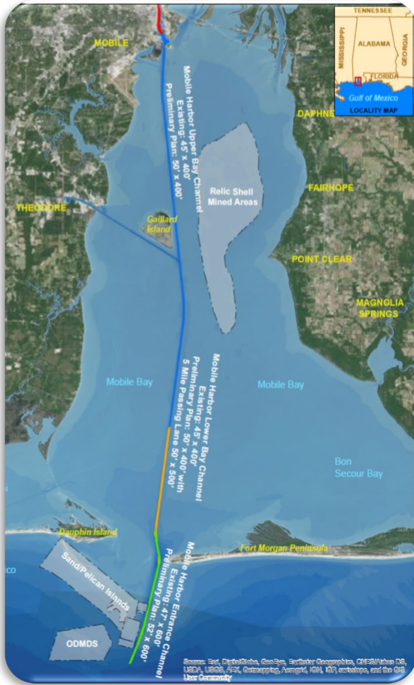
Figure 1.1 Overview of Mobile Bay within southern Alabama. The lines indicate the location of the navigation channel and proposed work location examined within the current report. Potential dredged material placement locations (not discussed herein) are shaded in grey.
