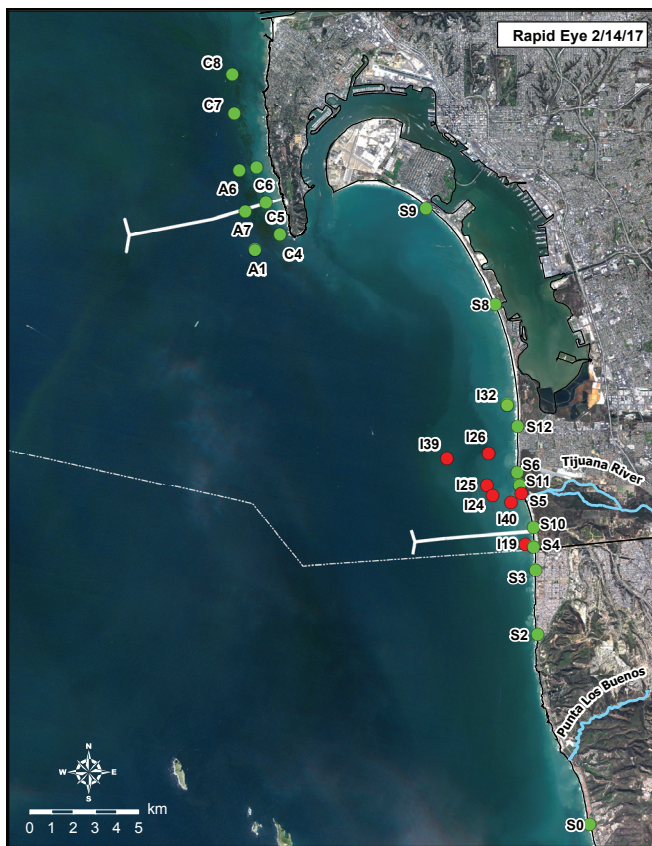
Figure 3.6 Rapid Eye satellite image showing stations throughout the region on February 14, 2017 (Ocean Imaging 2018) combined with bacteria levels sampled at shore and kelp stations on February 14, 2017. Turbid waters from the Tijuana River, San Diego Bay and Los Buenos Creek, can be seen overlapping stations with elevated FIB (red circles).
