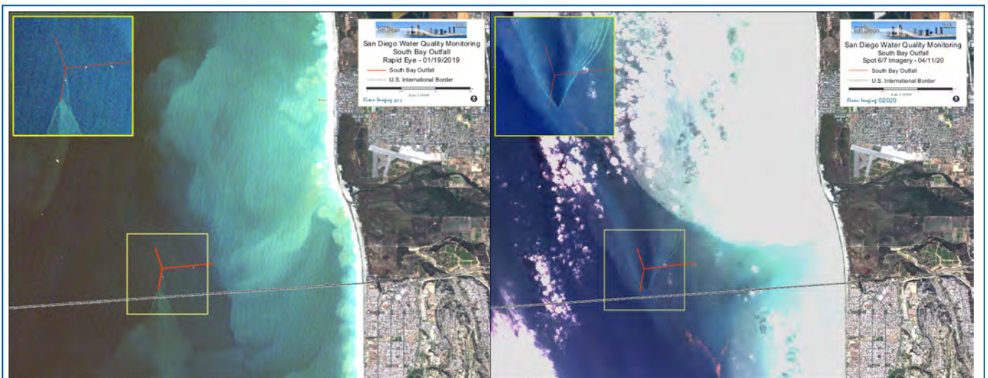
Figure 15. Examples of large SBOO effluent plumes at the oceans’ surface observed in a RapidEye image acquired on 01/19/19 and a SPOT image from 04/11/20 when the measured EFF TSS levels were relatively low (12.0 mg/L and 7.4 mg/L respectively).
