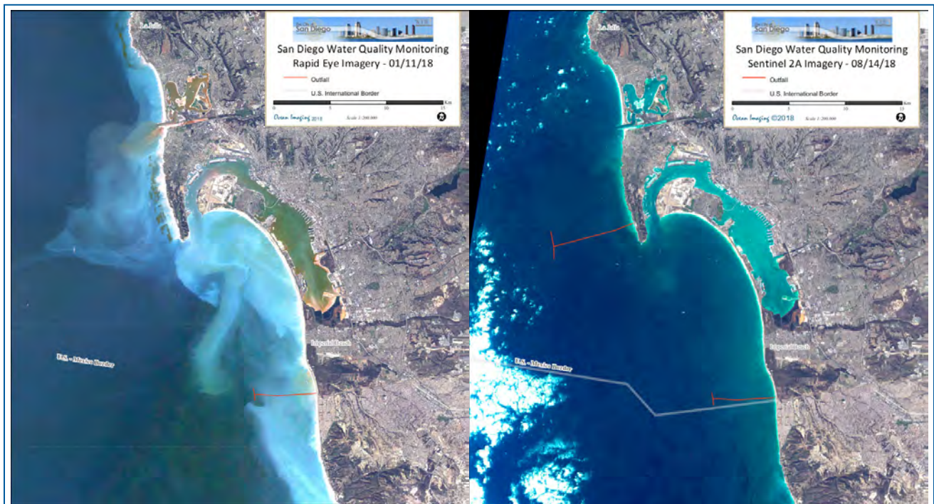
Figure 23. RapidEye image from 01/11/18 (left) one day after a significant rain event in which the strong San Diego River discharge is evident. In contrast the Sentinel 2A image from 08/14/18 exhibits the clear water conditions resulting from a near rain-free summer.
