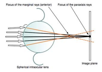
Longitudinal spherical aberration: difference of the distance between the marginal and paraxial rays.
