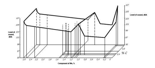
Figure - 4. Level of a sound of skilled steels in dependence from the carbon and manganese maintenance
