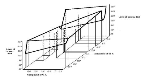
Figure - 2. Level of a sound of skilled steels in dependence from the carbon and silicon maintenance
