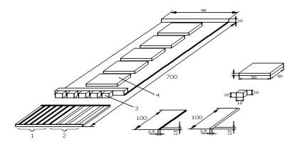
Figure - 1. The scheme of a cutting of samples for research:
