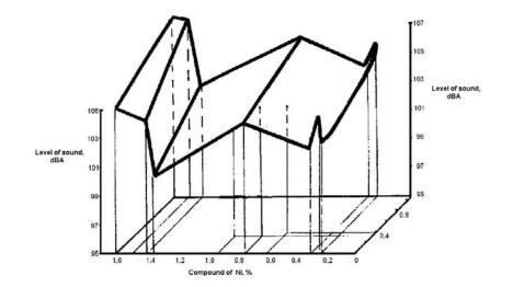
Figure - 6. Level of a sound of skilled steels in dependence from the carbon and nickel maintenance
