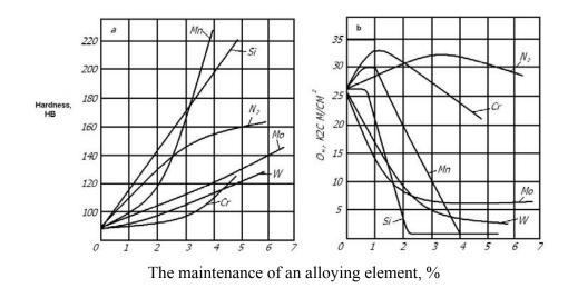
Figure - 5. Influence of alloying elements on properties of ferrite
