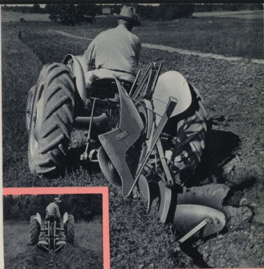
By lowering both right and left hand bases, you have a "V" plow for irrigation or drainage ditching.
