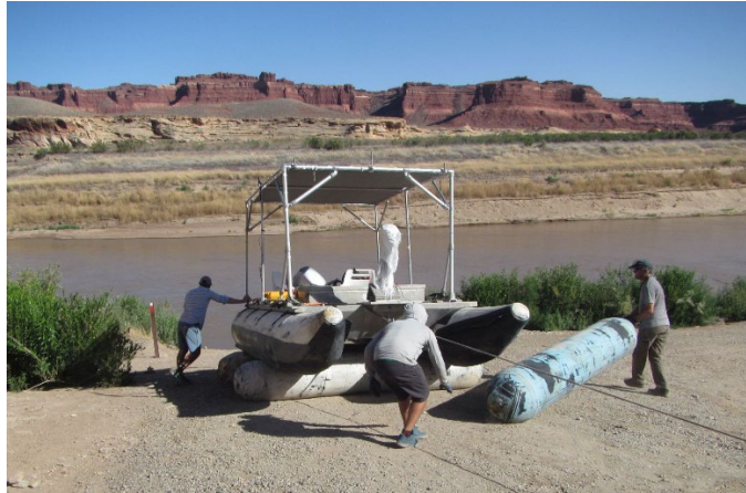
Figure 4. Launching survey vessel at North Wash boat ramp, about 900 m downstream from the mouth of the Dirty Devil River. The incising riverbed has caused the boat ramp to become too steep for safe use with vehicles and boats must be launched and retrieved by mechanical winch.
