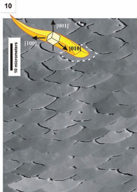
fig. 10. Perfect cross section through an array of fibrous calcite crystals of Megerlia truncata and a sketch indicating a typical fibre with its crystallographic orientation. Note the convex and concave sides of the fibres.
