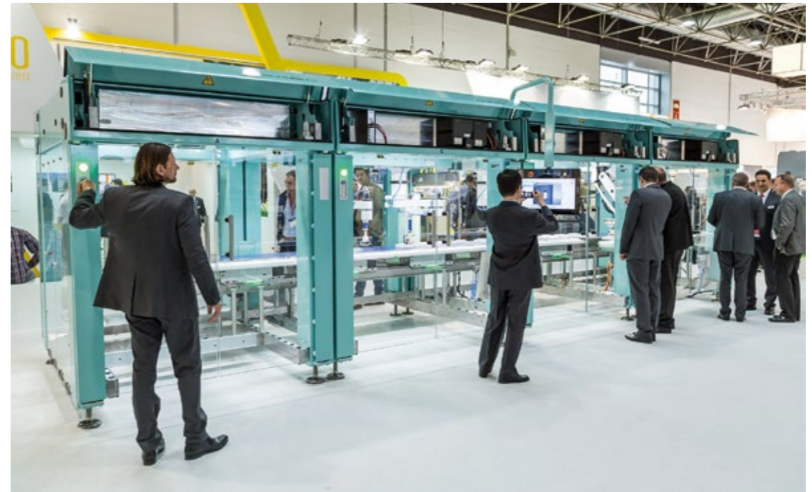
Packaging machine manufacturer Gerhard Schubert GmbH from Crailsheim, Germany, presented the world's first cabinet-free packaging machine during the interpack 2014 based on the drive system IndraDrive Mi.
