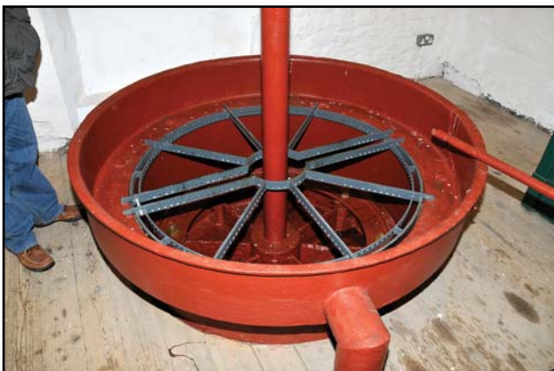
Left: The top of the Newcomen engine piston - fitted with a 'shield' to stop visitors falling.
