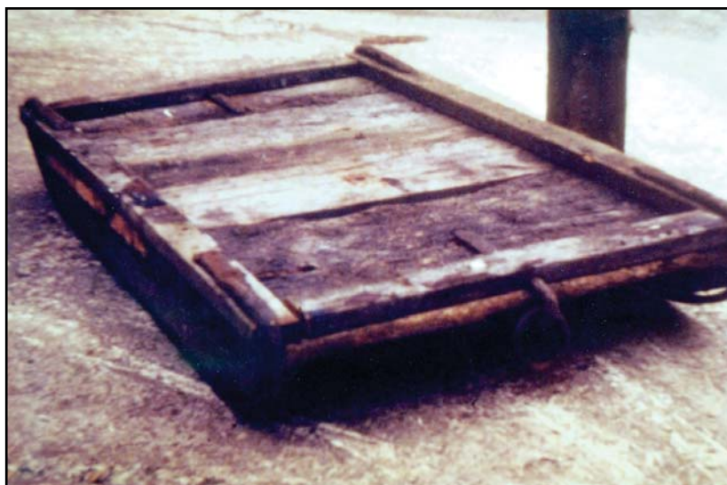
Below: The 1930s Sledge from Hanwood Pit. In operation a "square" timber frame was put on the sledge to carry more coal. (Ivor Brown)
