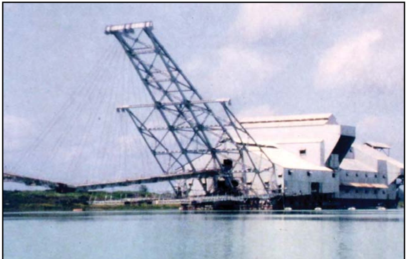
Above, 2: Tin dredger on a 1,000 acre site. 3,000 ton weight, 10ft. draught and 240ft. long bucket elevator. Large screen layout aboard, 200 men employed. Selanger Dredge Pit, Malaysia 1987. (Pictures: Ivor Brown)
