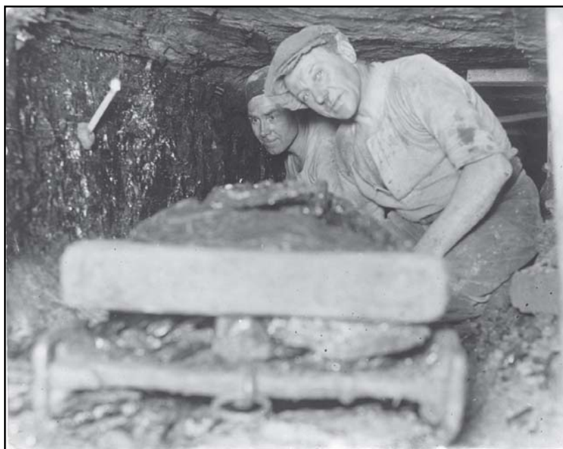
Above: Hanwood Colliery c1930. Two miners moving a sledge or 'dan' of coal. Miners: Percy Mansell (at the back) and Walter Challinor (at the front) near the coal face. A candle is stuck in a gob of clay on the coal face. (Howard Davies Shrewsbury Coalfield Collection)
