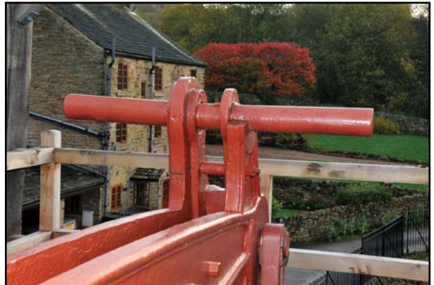
Below: The damaged catch-wings on the outside end of the Newcomen beam.
