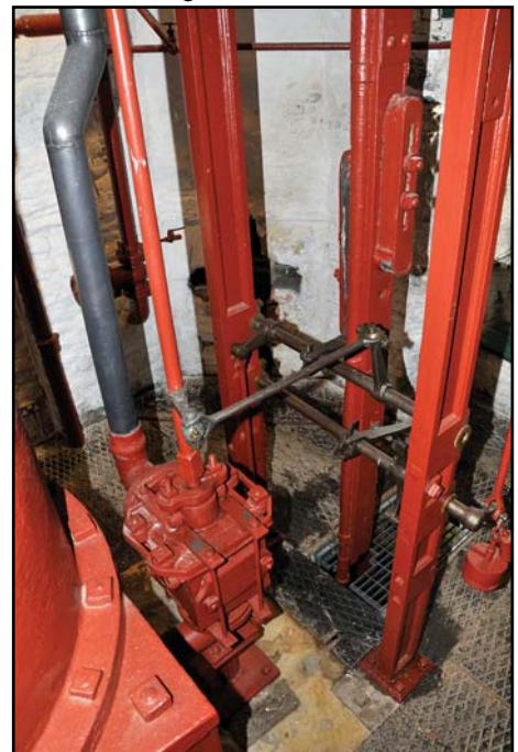
Below: The valve gear on the 1795 Newcomen engine.
