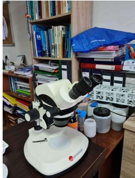
Figure 2: Stereomicroscopes for laboratory processing of samples
