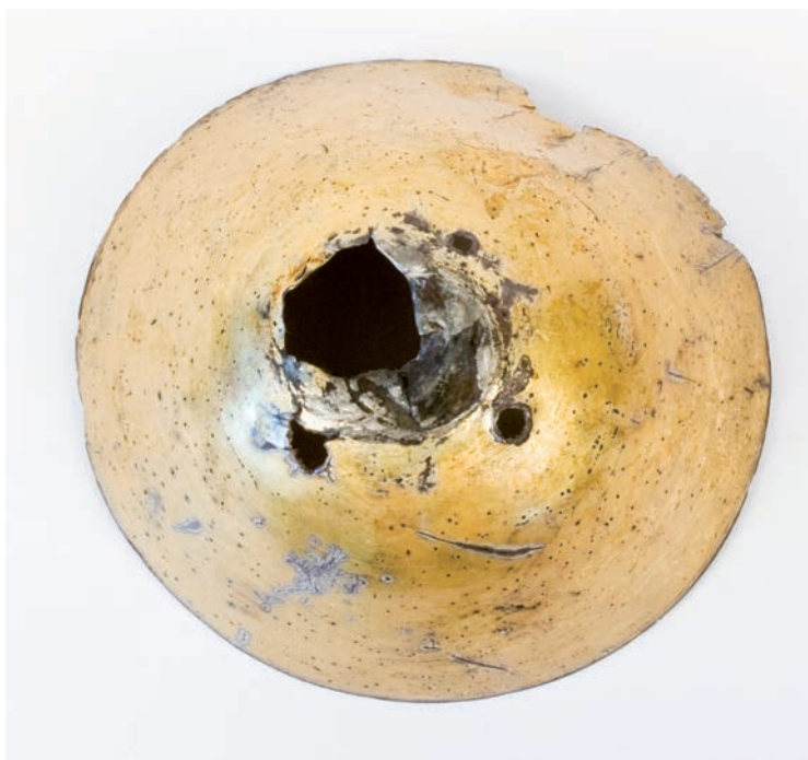
Fig. 38. Cup of the 14th-century communion chalice of Kökar Church. The broken cup and the remains of soldering mass on its bottom show how the stem was soldered on the bottom of the cup (Cat. 2:4).
