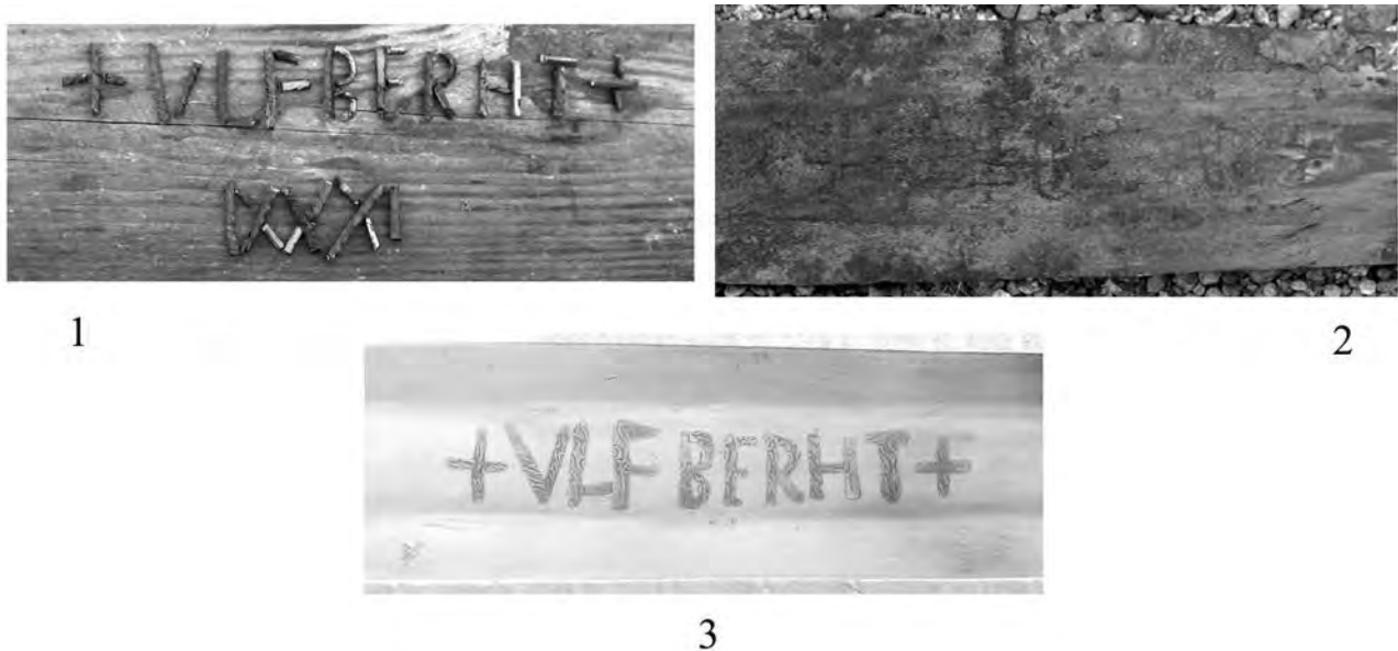
Fig. 5. Phases of the latest experiment: 1. Letters, which are formed from pattern-welded rods, 2. Hand-forged sword blade with welded inscription +VLFBERHT+, 3. The same blade polished and etched to enhance the inscription. Photos by Mikko Moilanen.
