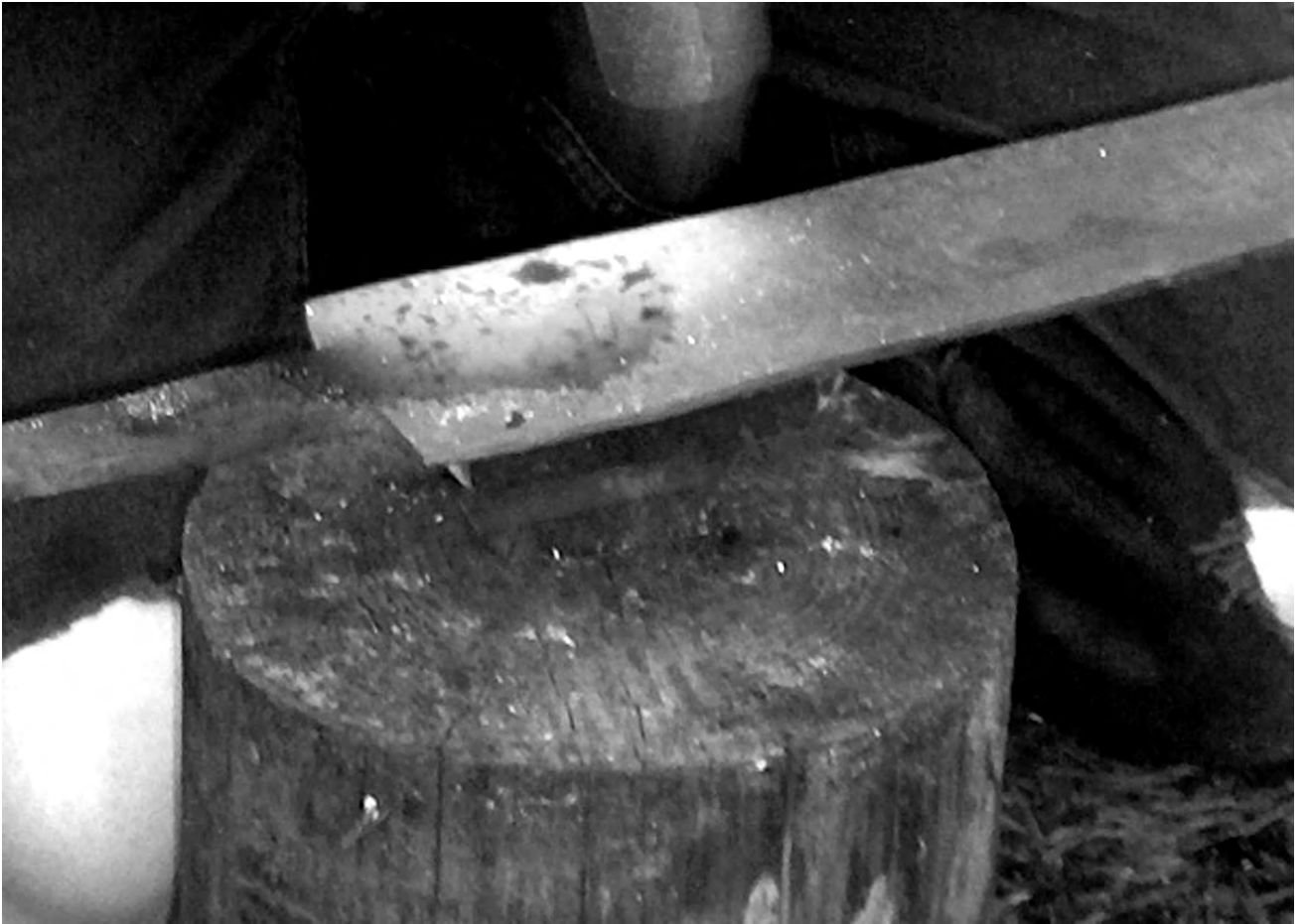
Fig. 4. A letter being hammer-welded onto the fuller of a half-finished sword blade. The anvil is relatively small and is attached to the wooden log, while the hammer is also quite small with a little convex face. The fuller of the blade is semi-finished until the letters are hammered in, at the same time deepening the fuller. Photo by Ulla Moilanen.
