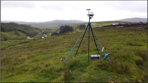
Plate 5-4: Anemometer and Rain Gauge
