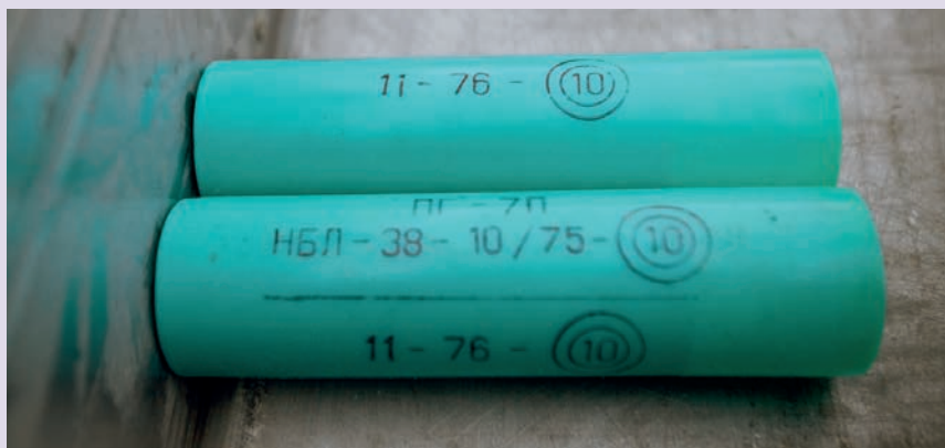
Image 5.53 PG-7P expelling charges for the RPG-7 shoulder-fired recoilless weapon
