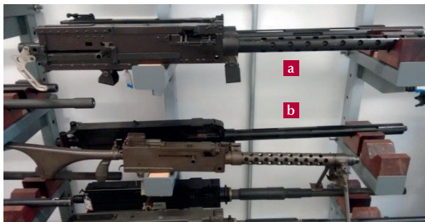
Image 5.22 A Browning M2 HMG and its close relative and small arms equivalent, the M1919A6
