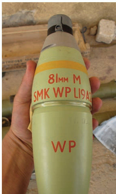
Image 5.45 Markings on a British L19A2 white phosphorous (WP) smoke 81 mm mortar projectile
