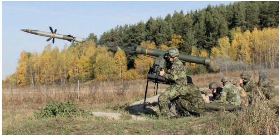
Image 5.21 A Swedish Saab RBS 70 NG CREWPADS firing BOLIDE ‘all-target’ SAM
