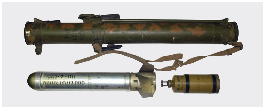
Image 5.50 An early Soviet RPO-A shoulder-fired 93 mm recoilless weapon showing the projectile and distinctive propelling charge below the gun
