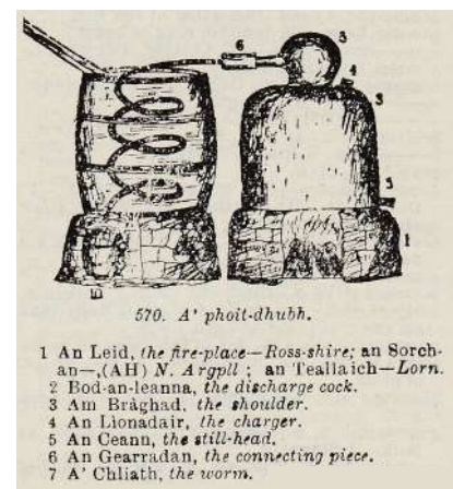
1 An Leid, the fire-place—Ross-shire; an Sorch-an—(AH) N. Argyll; an Teallaich—Lorn. 2 Bod-an-leanna, the discharge cock. 3 An Braghad, the shoulder. 4 An Lionadair, the charger. 5 An Ceann, the still-head. 6 An Gearradan, the connecting piece. 7 A' Chliath, the worm.
