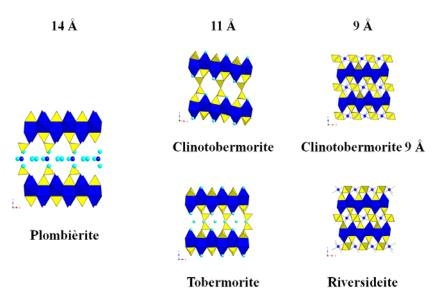
Fig. 2 - Crystal structures of the phases of the tobermorite group.
