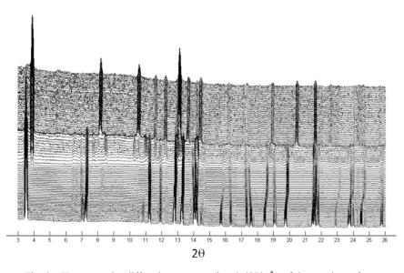
Fig. 3 - X-ray powder diffraction patterns ( $\lambda = 0.6873$  Å) of the specimen from NCIIM, from 25 up to 960°C.
