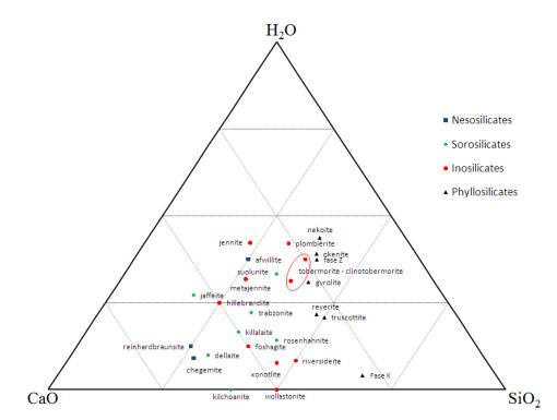
Fig. 1 - CaO-SiO<sub>2</sub>-H<sub>2</sub>O triangular diagram, showing the molar composition of C-S-H phases.
