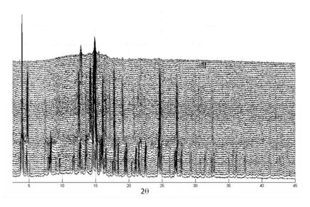
Fig. 5 - X-ray powder patterns ( $\lambda = 0.7835$  Å) of the specimen from Montalto di Castro, from 32 up to 843°C.
