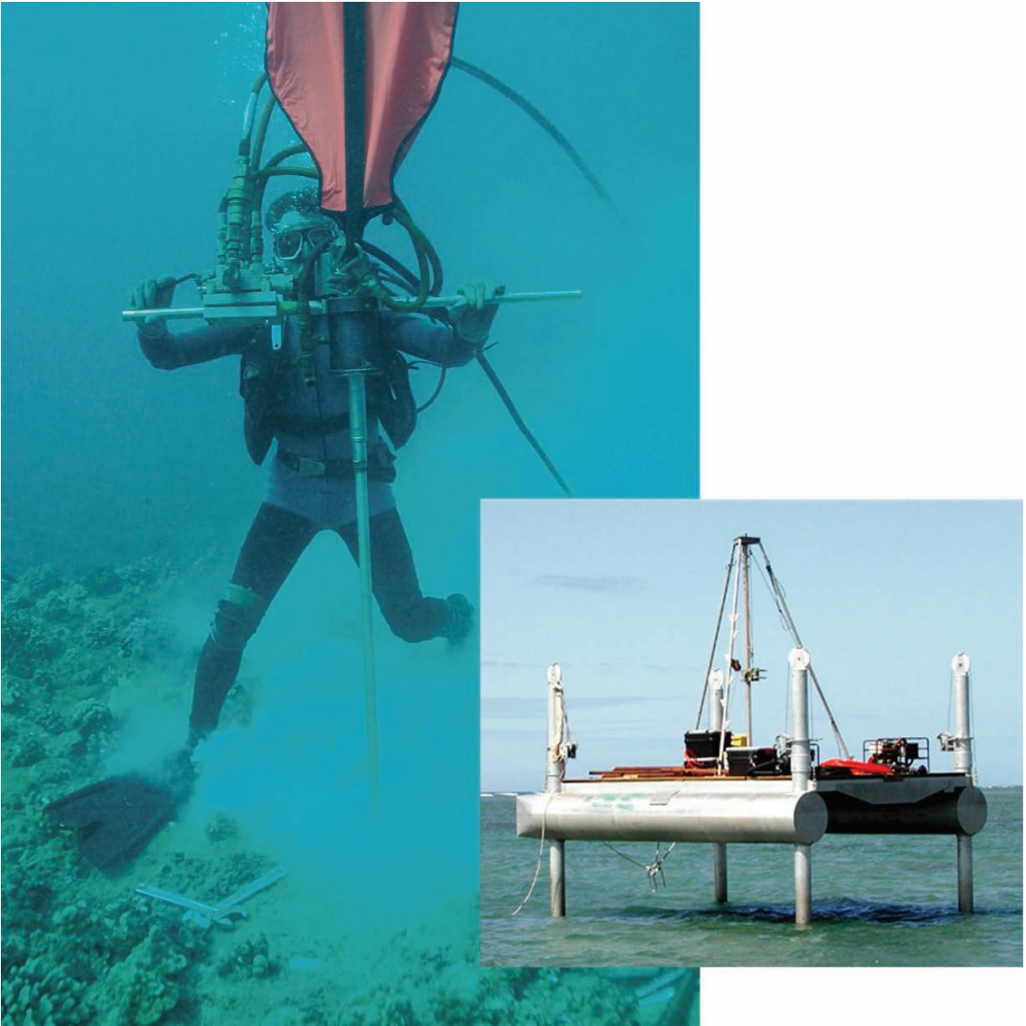
FIG. 11.18. Cored samples are obtained using both wireline and open-bit coring. The University of Hawaii jack-up drill barge provides access to shallow (<2m depth) reef sites
