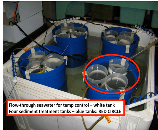
Figure 2. Sediment Treatment System. Four treatment tanks, each containing 3 of the larval chambers were inserted into a 4'x4'x2' temperature control tank.
