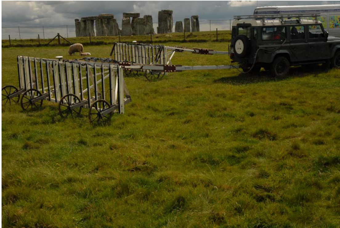
Plate 5 Multi-sensor vehicle-towed gradiometer at Stonehenge, June 2011. Photograph by Timothy Darvill. Copyright reserved: BU and DAI
